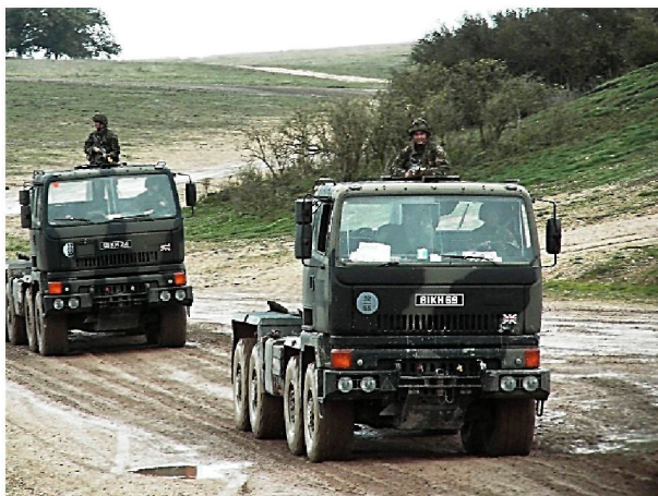
Above: 151 Transport Regiment Operating the Demountable Rack Offload and Pickup System (DROPS)
