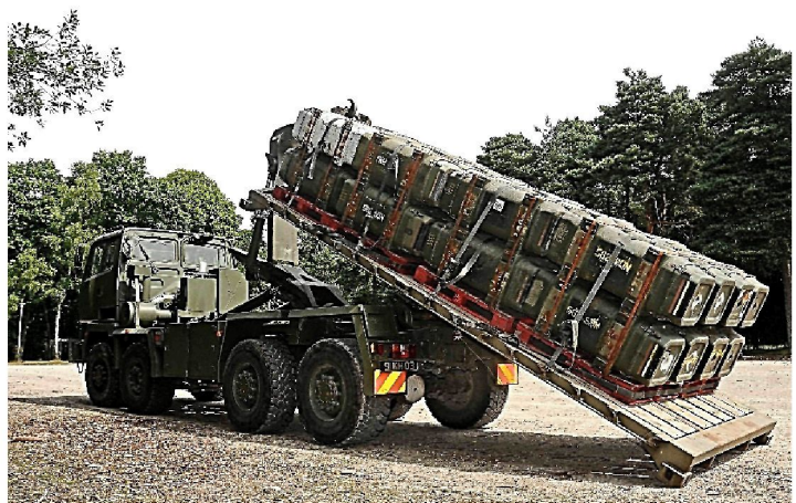
Above: 151 Transport Regiment Operating the Demountable Rack Offload and Pickup System (DROPS)
